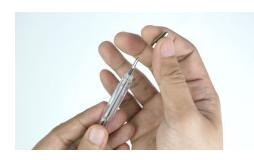
Remove the ink from a plastic pen to make a blow pipe
