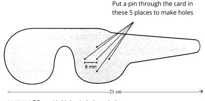
PICTURE 36 Multiple pin-hole occluder
