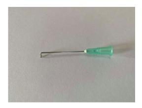
21 gauge needle with tip removed and end bent to 90 degrees
